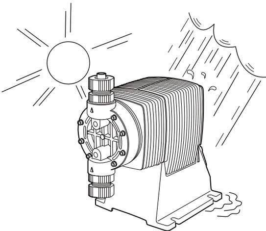
2. When installing pump, avoid the places where the pump is exposed to the direct sunlight, the ambient temperature is above 40 dig.C, or the relative humidity is above 85%. Though the pump has a simple waterproof and dust-proof structure, it is recommended to protect the pump with a cover when installing it outdoor.
