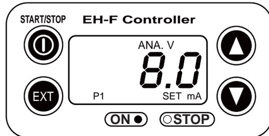
(5) Pushing EXT key once, "spm" appears on the display while "mA" disappears. The picture below shows the number of strokes at "P1".
