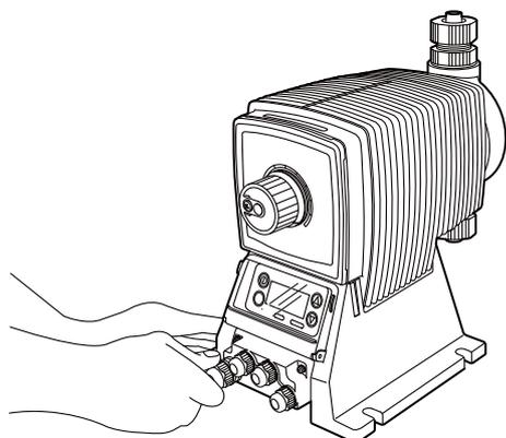
8. Fit and tighten a cord nut in the last place.
