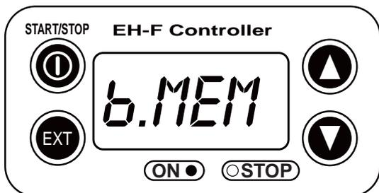
(6) Push EXT key in order to display the current set state. "SET" indication appears. The picture below shows the buffer memory is set to OFF.
