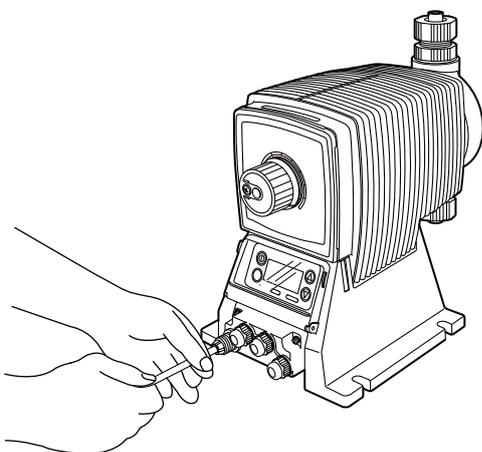
7. Adjust the slackness of cord in the terminal box and fit a cord gasket to into the terminal box.
