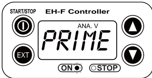
(2) Pump start to run at full speed when ▲ and ▼ keys are pressed at once. Display shows "PRIME". If either ▲ or ▼ key is released, pump returns to the previous mode. In this case pump returns to ANA.V mode.
