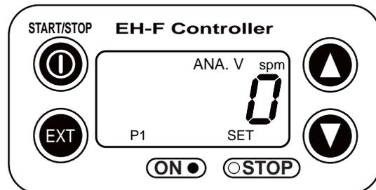
(6) Set the number of strokes at P1. Figure increases/decreases as ▲ / ▼ key is pushed. Picture below shows 10 spm is set for point 1.
