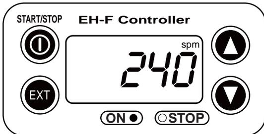
(2) ANA.V indication appears and pump enters an EXT mode as EXT key is pushed once. Pump starts operation in accordance with current signals and various settings. ON lamp blinks at each pumping during operation. Pump is controlled via the EXT mode which was selected at USER mode. The initial setting of EXT mode is ANA. V mode. Select a preferable EXT mode in USER mode. The picture below shows ANA. V mode. (The spm on the display changes according to input signals.)
