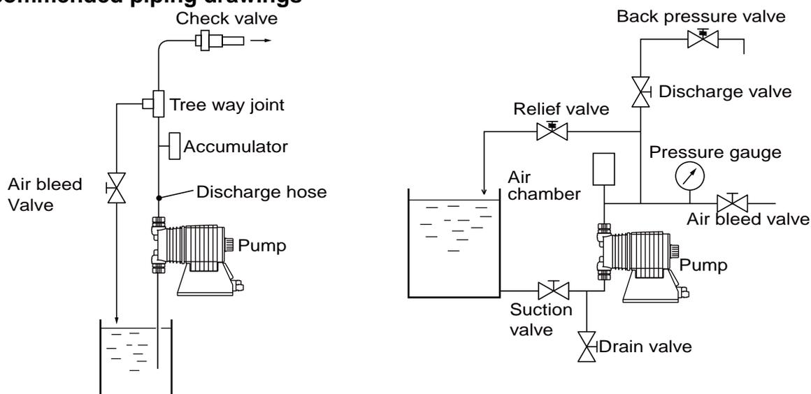
Arrange piping to meet the suction and discharge requirement. Especially pay attention to piping arrangement in case of handling the slurry which has settling property.
