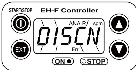
(1) In case Input signals fall to 4 mA or below while 4-20 or 20-4 is set to ANA. R mode, pump stops with "DISCN" blinking and "Err" on display.
