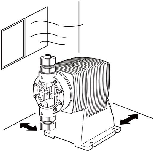
3. Select a level floor and use the four M6 bolts to firmly anchor the pump so as not to allow any vibration. If the pump is inclined, the discharge amount may decrease considerably.
