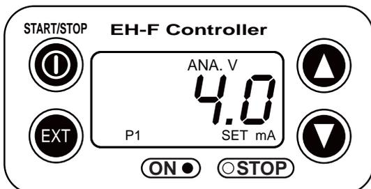
(4) Set the current value at P1. Figure increases or decreases as ▲ or ▼ key is pushed. The picture below shows 8.0 mA is set to point 1.
