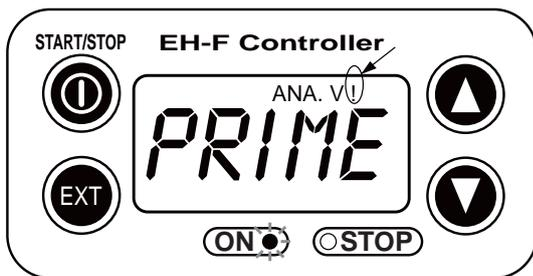
(3) Pressing both ▲ and ▼ keys simultaneously for 10 seconds or more, pump continues to run at full speed even if both keys are released. In this case "!" indication appears. Push either ▲ or ▼ key to release this state. "!" indication disappears and pump returns to the previous mode. In this case pump returns to ANA.V mode.
