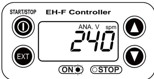
(3) Push EXT key once when pump is running in ANA. V mode. Display indicates the setting display of ANA. V mode. "spm" indication disappears, and "P1", "SET" and "mA" indications appear on the screen.
