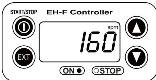
(2) This error state can be released by pushing START/STOP key and pumps enters wait mode. In this case check the wiring and input signals.
