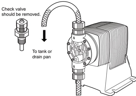
[1] Extend the tube connected to the discharge-side fitting out of pump to a chemical tank or a drain pan. Then start pump operation.
