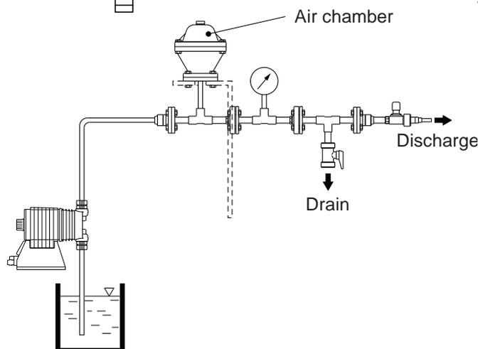
7. Accumulator and air chamber mounting.
